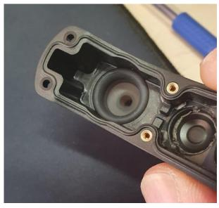
When reassembling the controller, please take care that the sub-boards carrying the buttons are properly seated in the recesses in the main PCB or the enclosure will not come back together.
